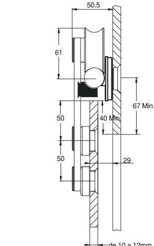
SOPORTE PERFIL PARED / Wall support profile / Support du rail sur mur.
